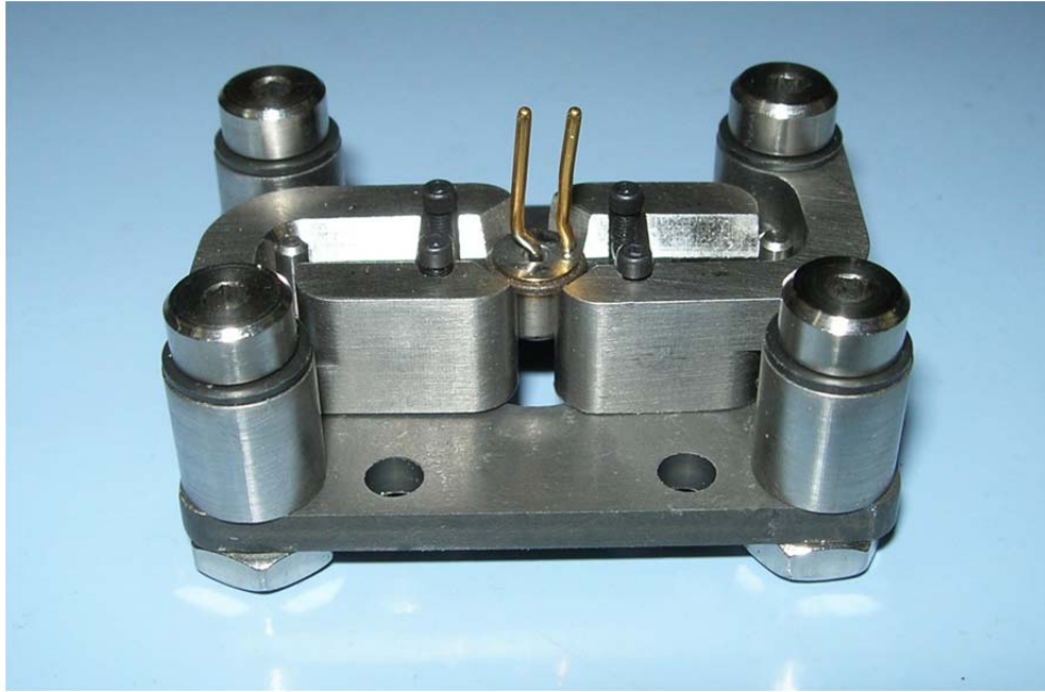
Figure 6: Unmolded header in production line tooling
