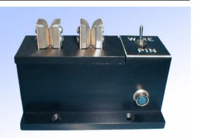
Dedicated Kelvin connectors for leadwire parts. These mountable connectors are designed with precious metal plating overbrass or Elkonite contact material for very long life and high accuracy. A unique'S'shaped innerprofile assures repeatable measurements with small gage or stranded wires.
