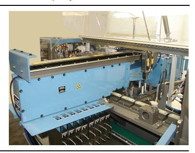
A variety of x-ray sources are available, including those from Hamamatsu (80KV) and Kevex (130KV). This high speed station may be specified with image archive (DVD-RAM) or hard disk storage for different requirements. A separate image monitor is provided for real-time image display during operation.
