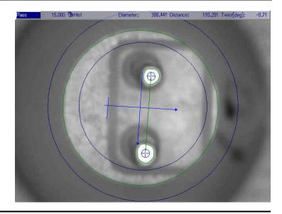
The vision option is a fully integrated camera system on the FET-C. This high speed station may be specified with PLC (discrete I/O) or computer (Ethernet) interface for different requirements. An image monitor is provided for real-time image display during operation.
