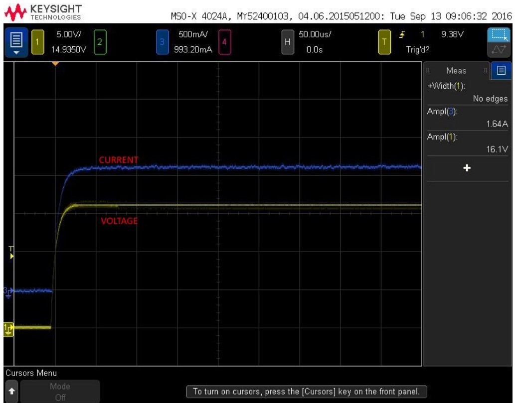
Figure 8: Rise time; voltage mode, 100ms, 16 volt pulse into a 10-ohm load
