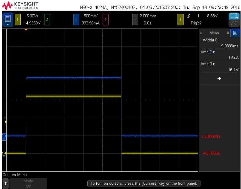
Figure 4: Voltage mode; 10 millisecond, 16 volt pulse into 10-ohm load
