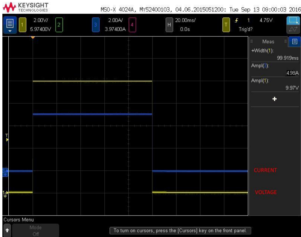
Figure 3: Voltage mode; 100 millisecond, 10 volt pulse into 2-ohm load
